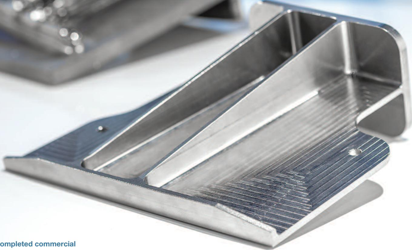
**Completed commercial aerospace titanium part next to its near-net RPD form.**
