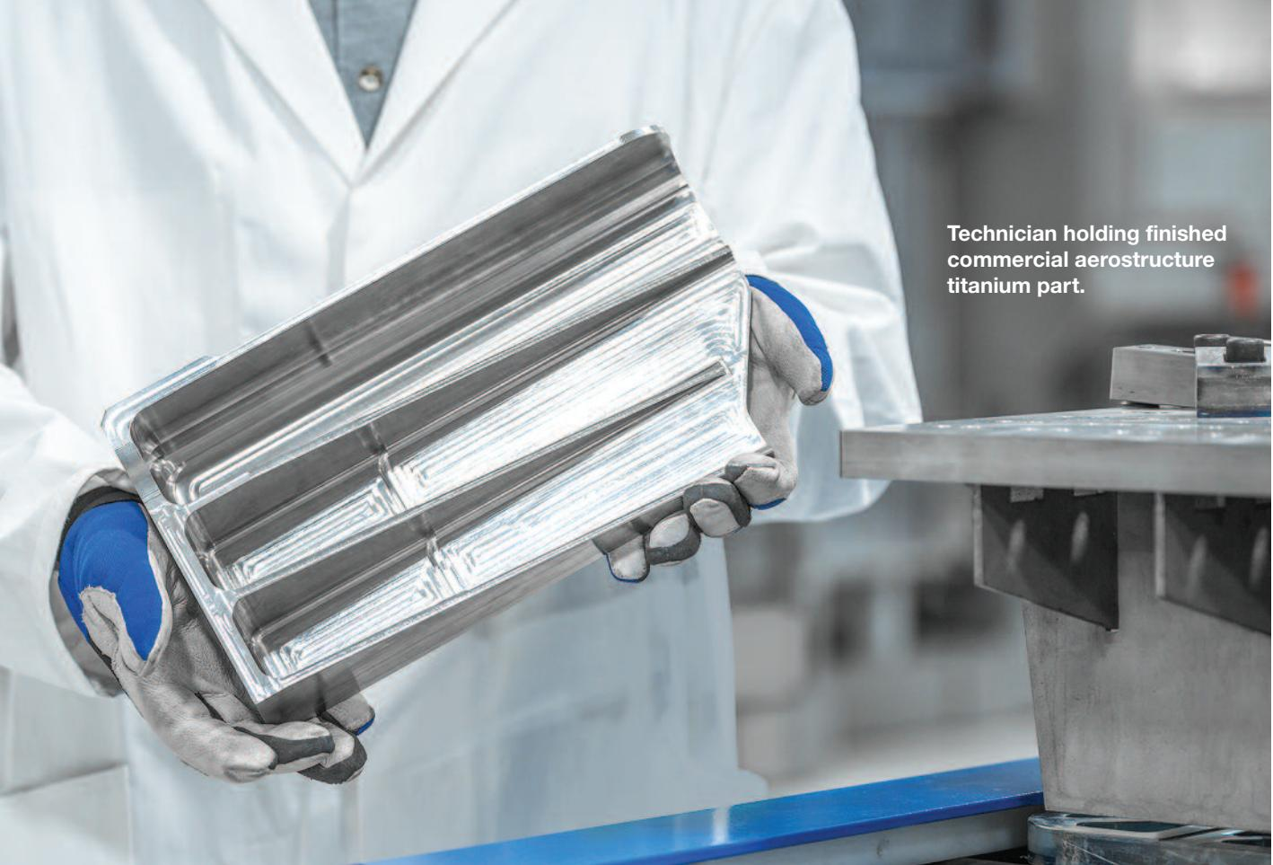
Technician holding finished commercial aerostructure titanium part.
