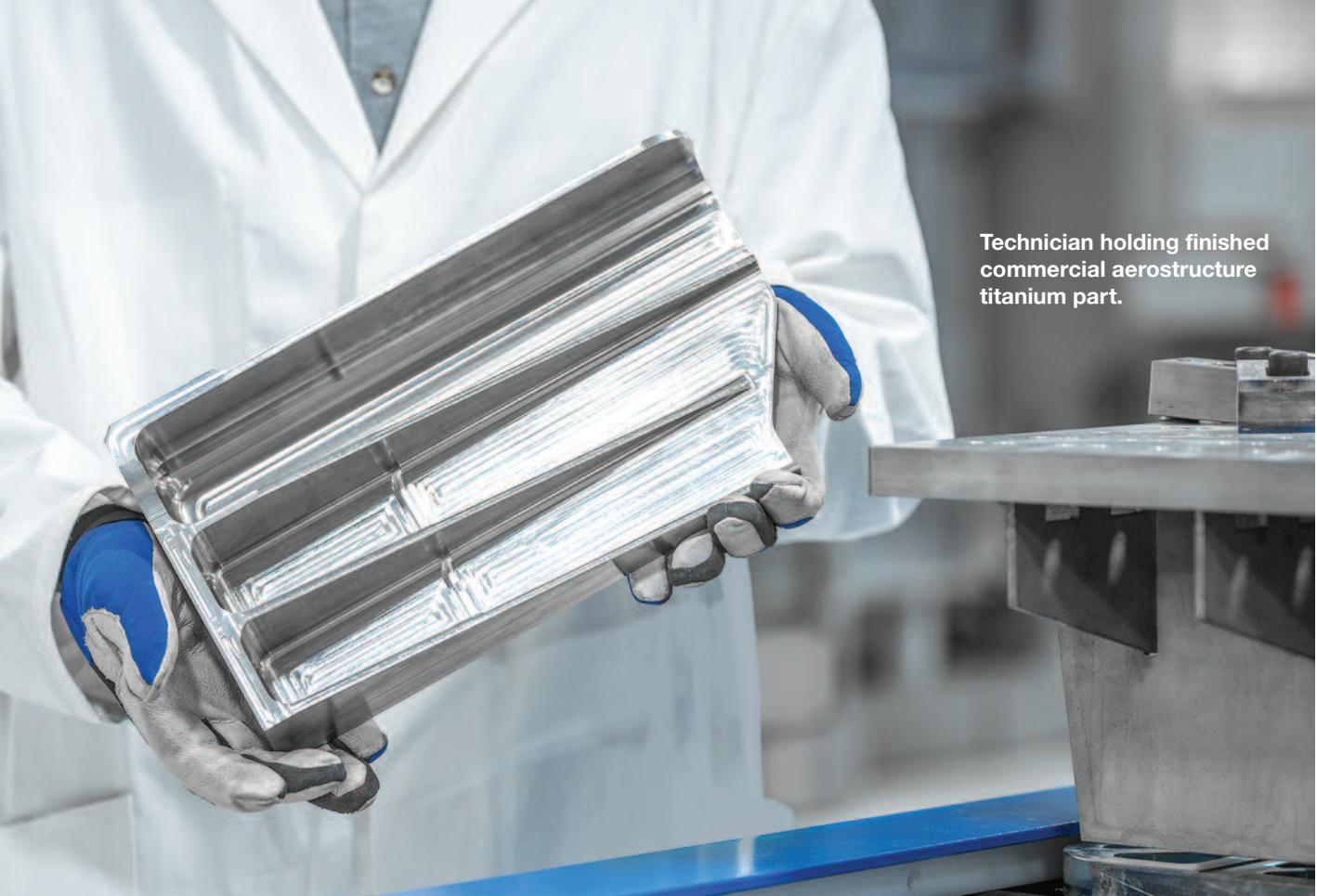
Technician holding finished commercial aerospace titanium part.
